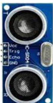
Figure-4: An ultrasonic Sensor
